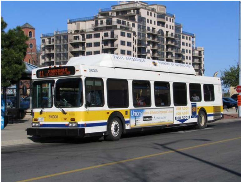
New Flyer bus with Cummins Westport C Gas Plus engine
